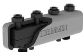
5539X Insulated steel hydraulic/ manifold separator and fixing brackets, circuit centre distance 125 mm, connections with flat seat and 1"1/2 cap
