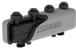
5539X Steel hydraulic separator/ manifold with insulation shell and fixing brackets, 125 mm circuit spacing, 1"1/2 fittings with flat seat and cap
